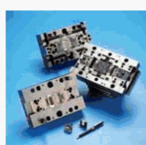
Micro tools can accommodate two-shot molding. Makuta uses this shuttling mold to produce a small ABS part with raised lettering in a second color. The letters are only 0.25 mm wide.
