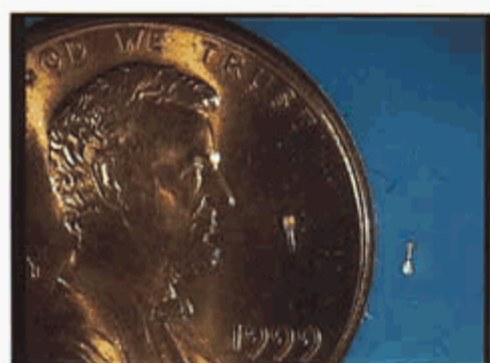
This is the world's smallest production part. It is ejected with a .0050-inch diameter ejector pin. Images courtesy of Miniature Tool & Die.
